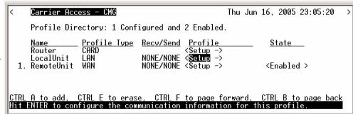
Profile Directory Window 3. Select **Setup: <Secondary IP Address>**, by scrolling through the options with the **[SPACEBAR]** and select **[ENTER]**. Select **[CTRL A]** to enter an IP Address.
